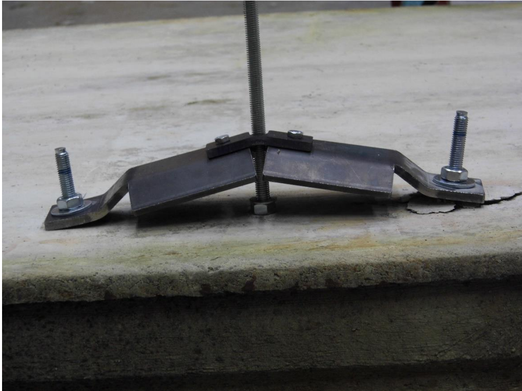
Figure 5. Typical failure mode for all specimens except specimen 2
